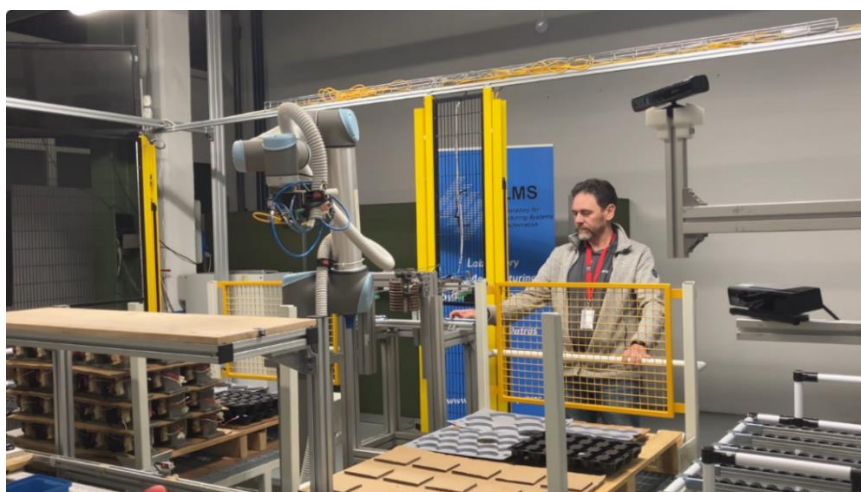
Figure 112: Safety verifications the robot must change to collaborative speed when light barriers are triggered
