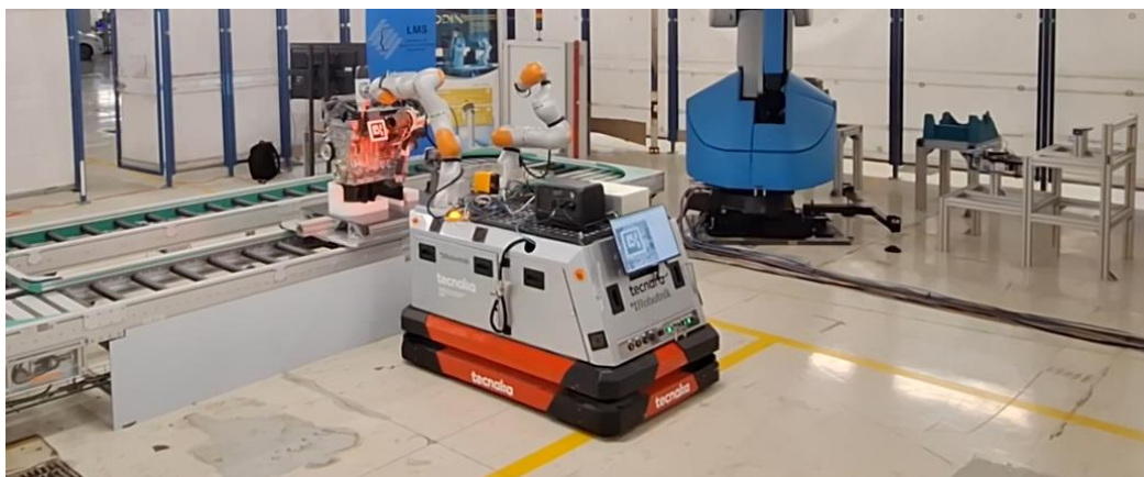
Figure 47: Mobile manipulator fastening screws on moving engine
