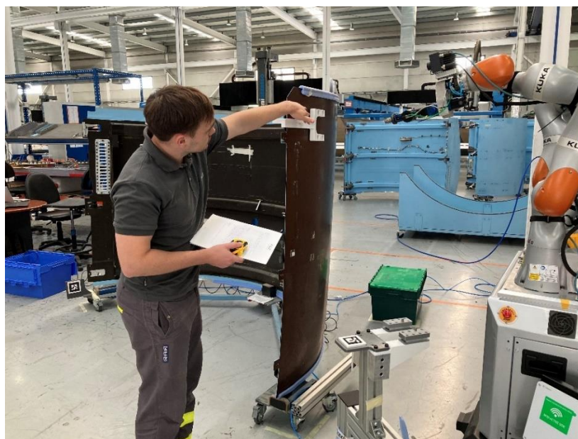
Figure 81: Safety areas distance verifications
