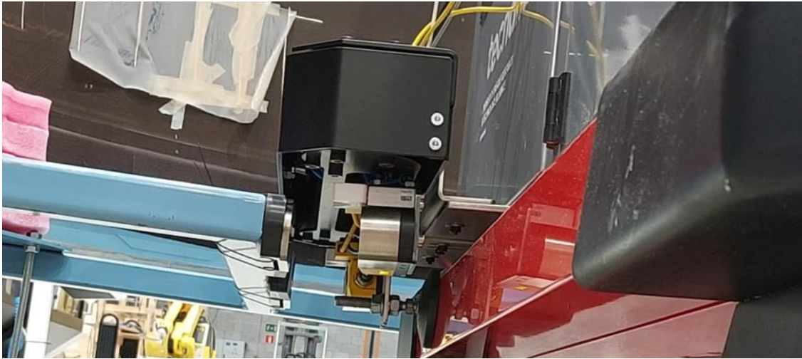
Figure 63: Magnetic docking for fan cowl transportation in the robot
