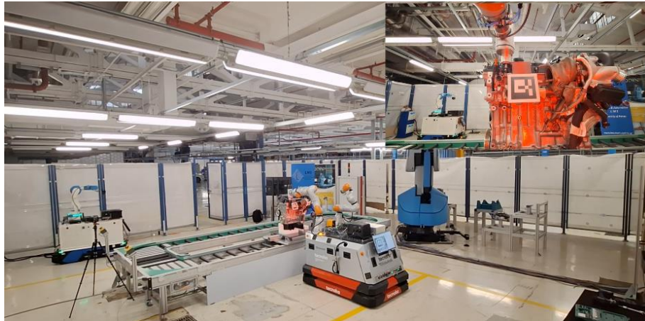
Figure 13: TECNALIA robot performing the screwing while moving task
