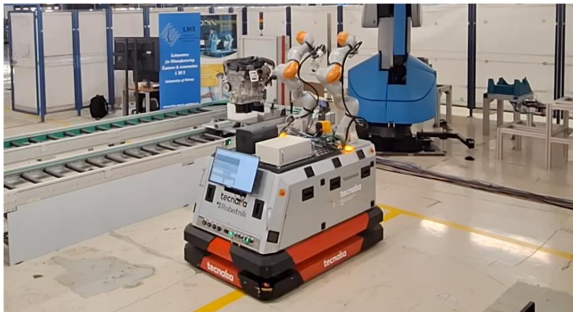
Figure 11: TECNALIA mobile robot navigation to the motor and gearbox assembly area
