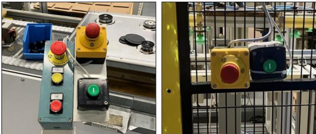
Figure 114: Emergency stop and reset buttons integration
