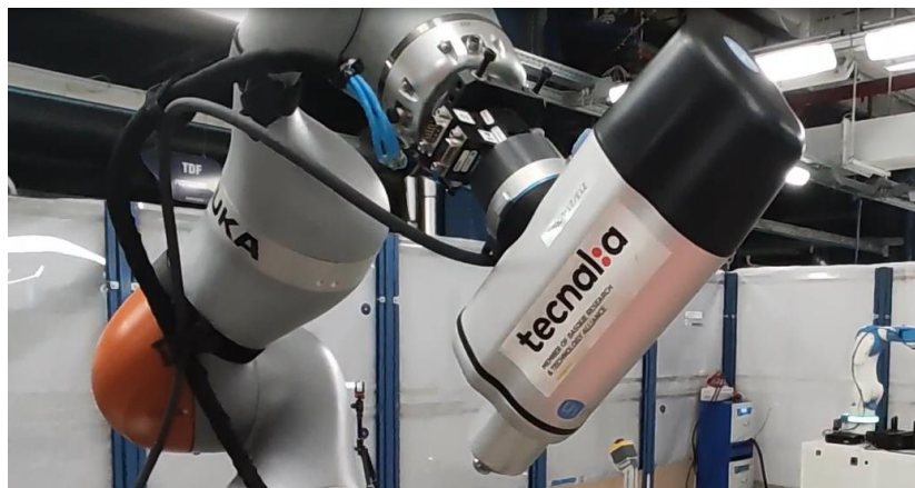
Figure 9: OnRobot automatic screwdriver used for screw fastening
