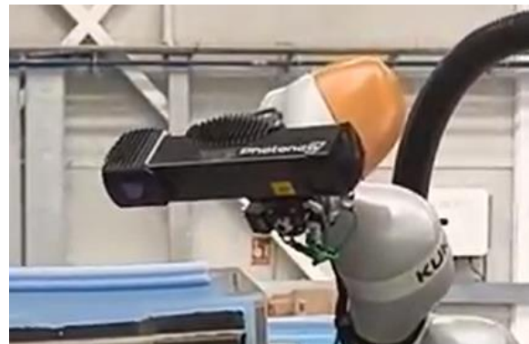
Figure 66: Photoneo MotionCam-3D mouter on right arm
