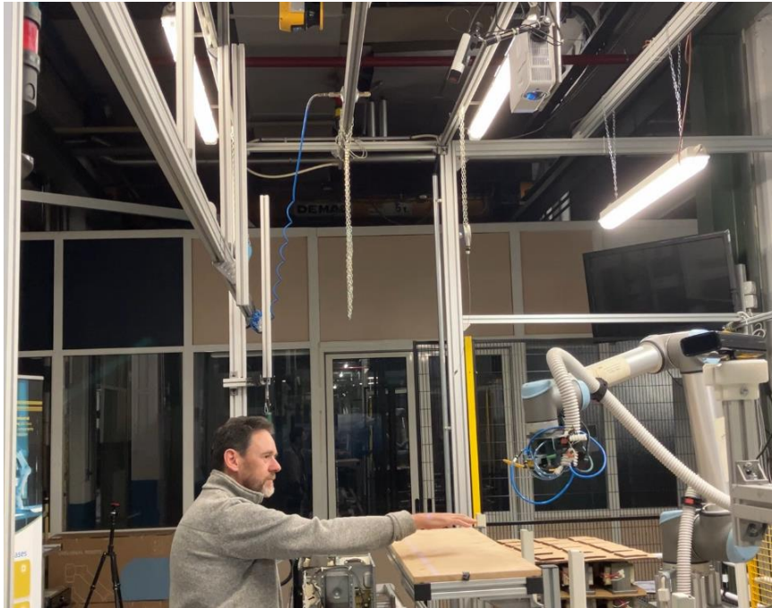
Figure 117: Safety verifications to reduce the speed of the robot when human operator triggers the safety zone of the scanner
