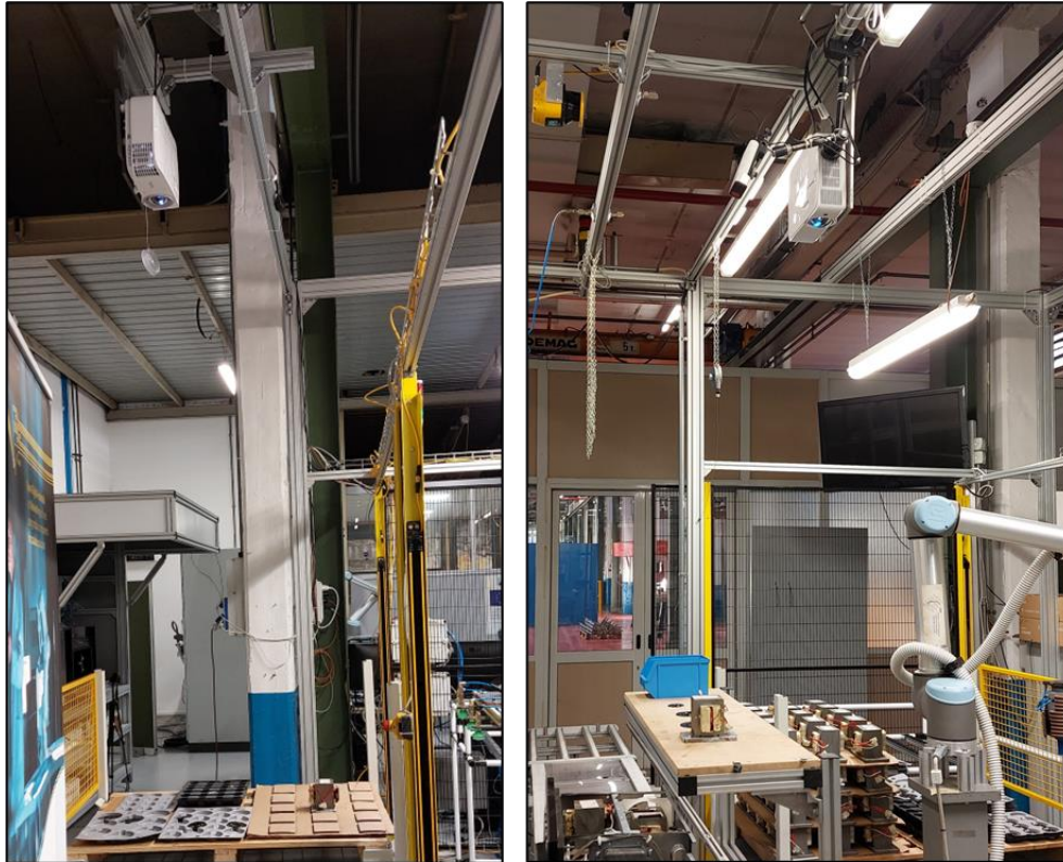
Figure 95: a) Projector at the back of the work cell, b) projector and Kinect camera at the front of the work cell
