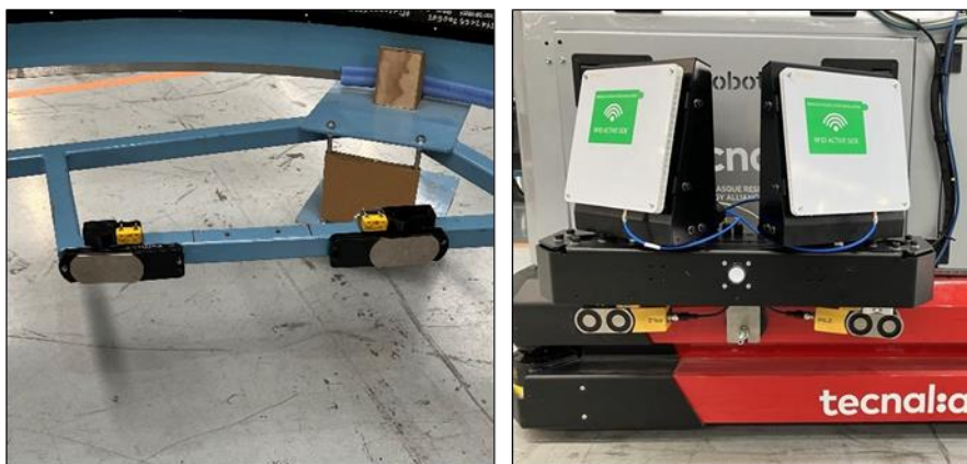
Figure 83: Magnetic sensor used for attaching the fan cowl to the mobile platform
