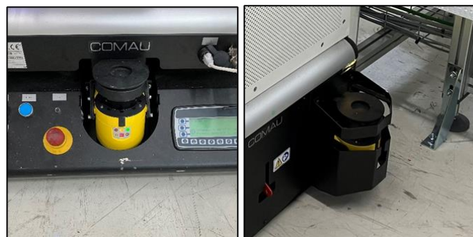
Figure 44: COMAU safety laser scanners
