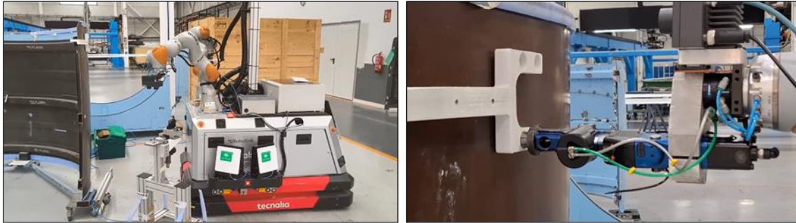
Figure 57: Execution of drilling operation at AEROTECNIC premises
