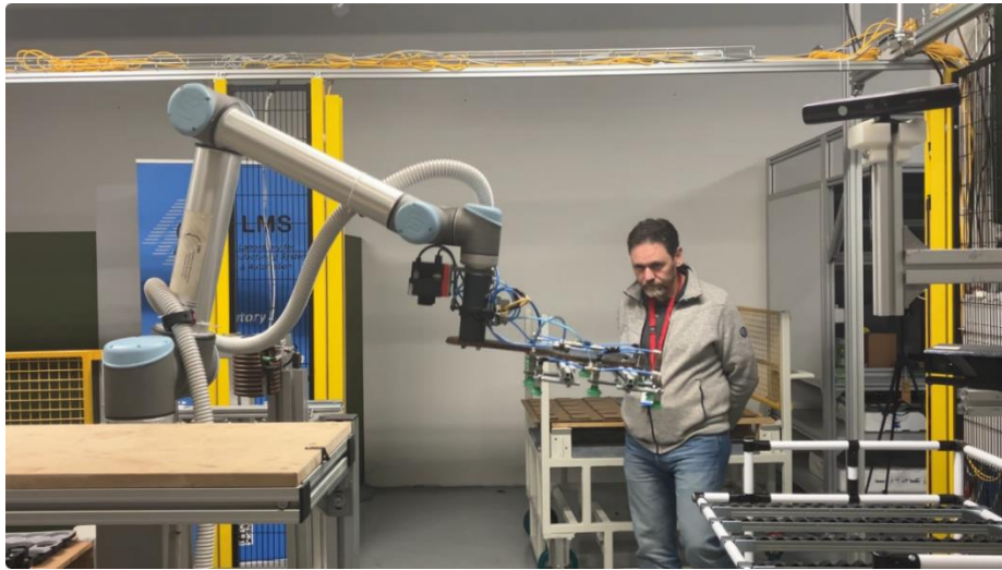
Figure 113: Safety verifications where the robot must immediately stop if attached to the robot is the pneumatic gripper and the light barriers are triggered
