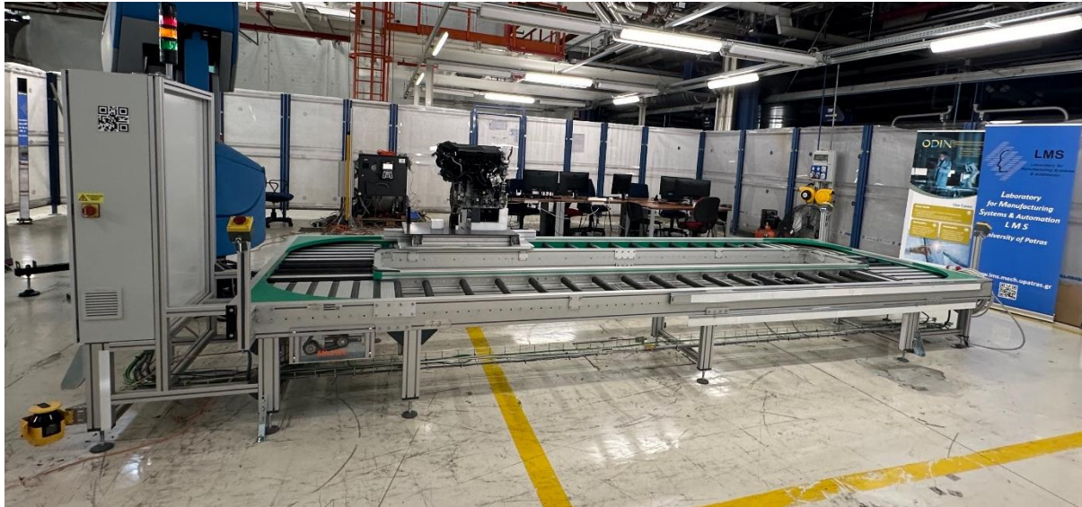
Figure 6: Installation of movable conveyor at STELLANTIS premises
