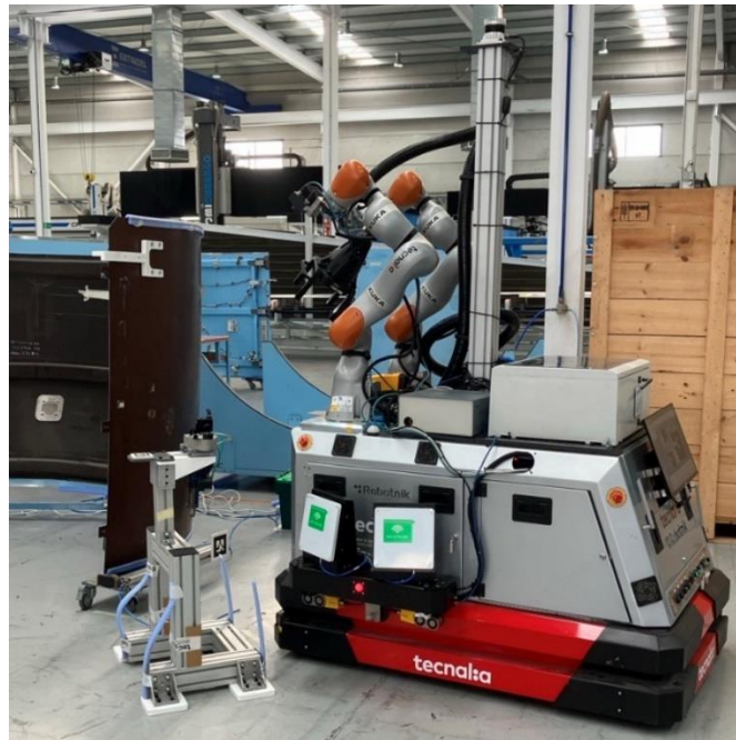
Figure 80: Mobile platform in drilling position
