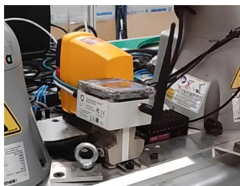
Figure 42: Wireless safe bridge to communicate with the external safety manager
