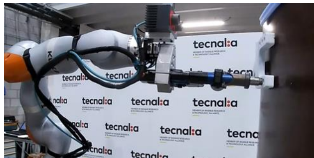
Figure 62: SETITEC ST1200 driller attached to the left arm
