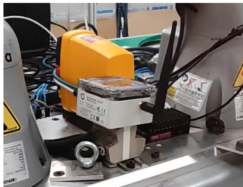
Figure 10: Wireless safety bridge to communicate with the cell's safety manager
