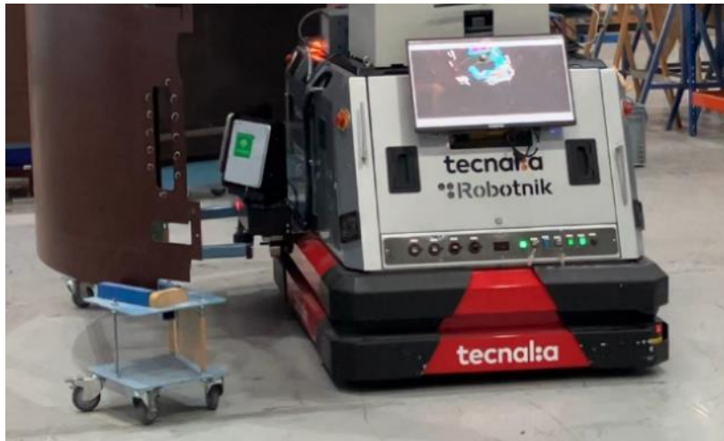
Figure 84: Emergency stop due the detachment of the safety magnetic sensor
