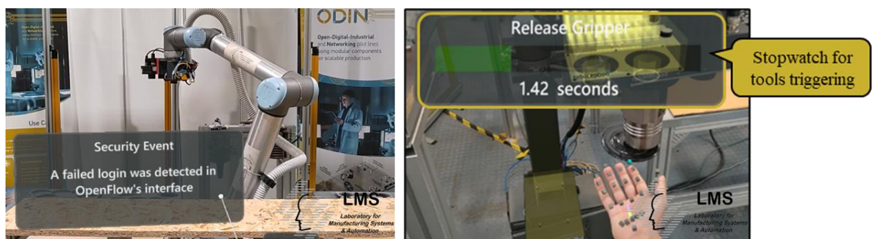
Figure 72: AR operator support application in White Goods pre-industrial demonstrator
