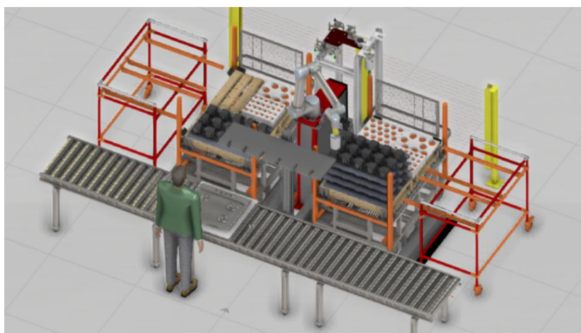
Figure 78: White Goods pilot demonstrator design for installation at WHEMAN premises
