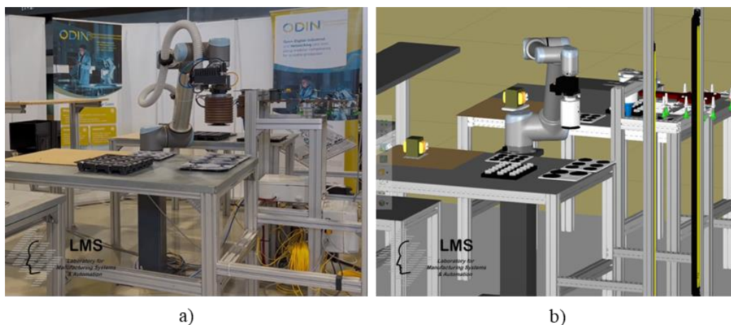
Figure 81: Virtual commissioning validation in the White Goods pre-industrial demonstrator
