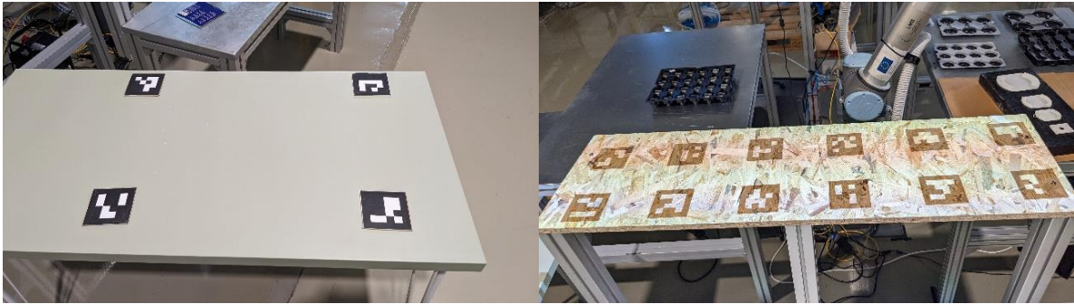
Figure 74: The display zone for the smart user-interface on mobile table (Left) and for the static borders (Right) are defined, with the help of ArUco markers.
