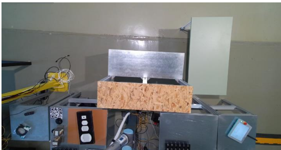
Figure 75: Scene from the Azure Kinect for the LMS White Goods test setup. Self for the assembled components in the centre. Mobile table for mobile projected UI at right.
