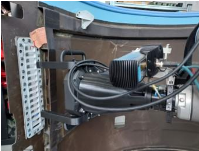
Figure 35: Integration tests with Keyence sensor
