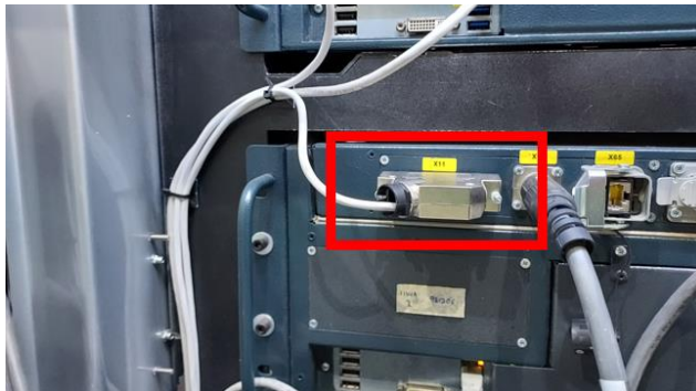
Figure 42: KUKA IIWA X11 connector where safety signals must be wired
