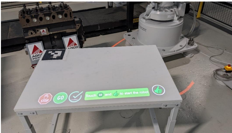
Figure 57: The smart interface is displayed on a table. The operator can interact with the displayed elements and control the robot operations.
