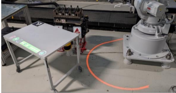
Figure 58: Red dynamic safety line projected around the robot.
