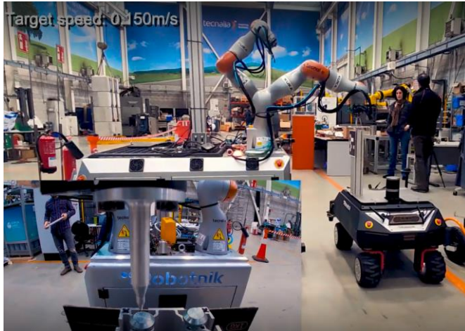
Figure 29: Target following tests at 9m/min
