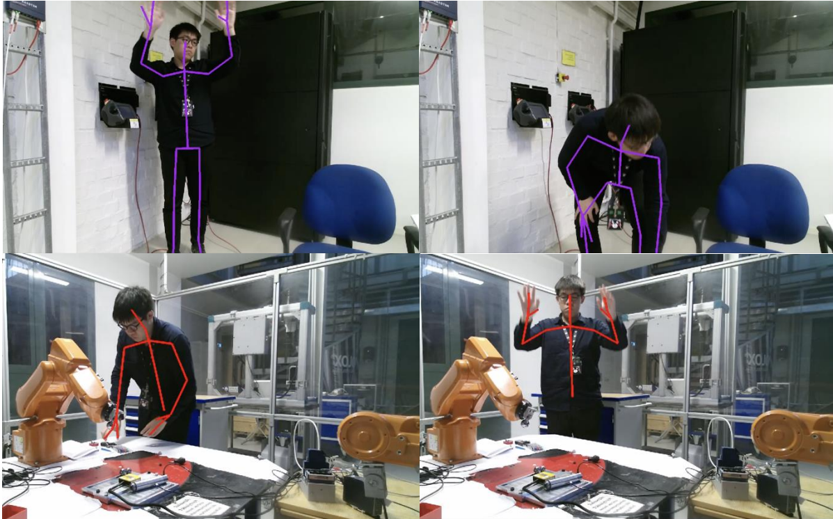
Figure 41: Some results of Kinect V2-based human body skeleton detection in KTH small-scale pilot.
