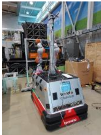
Figure 6: 3D LiDAR mast mounting with tightening cables
