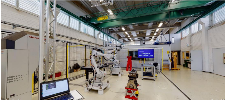
Figure 40: TAU's HRC environment used for ODIN – engine placed at the front of one ABB robots
