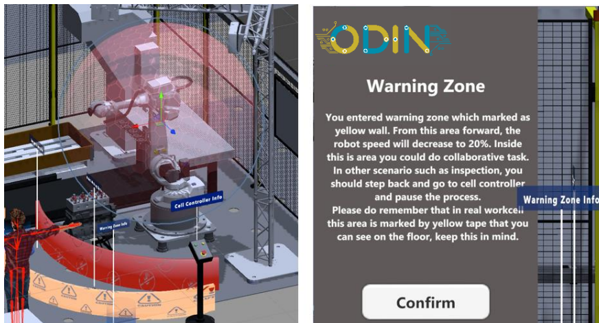
Figure 32: robot workspace representation in sphere shape (left), information of warning zone for operator (right)
