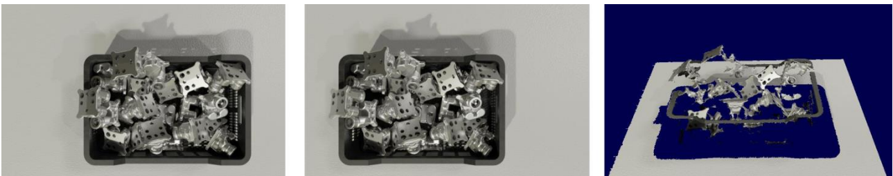
Figure 17: Simulation left and right stereo image pairs and reconstructed realistic point cloud
