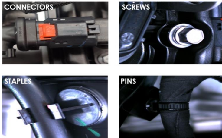
Figure 50: Sample parts on the Automotive engine used for the quality inspection evaluation
