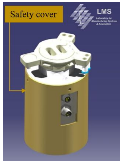
Figure 74: Safety cover for magnetic gripper
