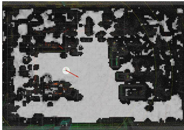
Figure 57: 2D transitivity map obtained from the elevation map
