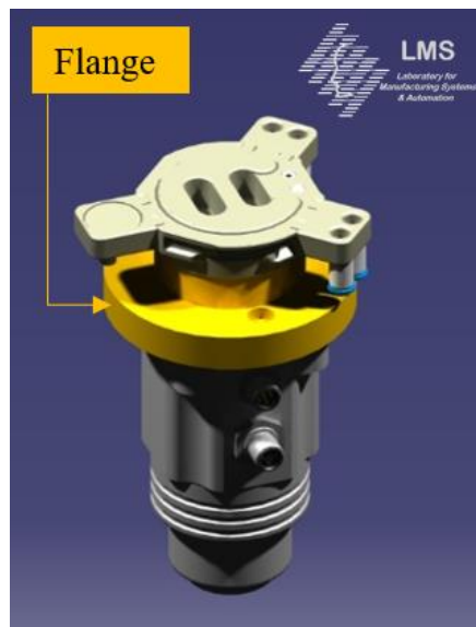
Figure 73: Flange for magnetic gripper
