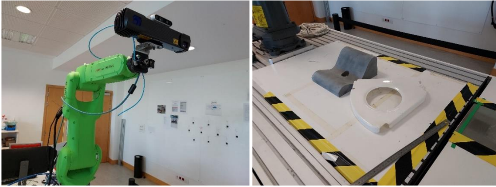
Figure 25: 3D vision sensor in eye-in-hand configuration (left) and workspace setup for reconstruction (right)
