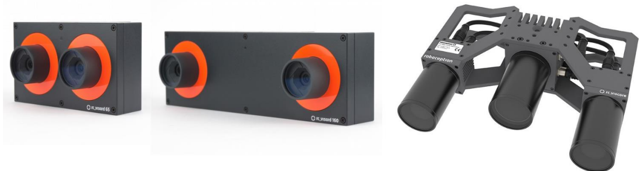
Figure 20: Stereo 3D vision sensors from Roboception tested with the object pose estimation software: rc_visard65 (left), rc_visard160 (center), rc_viscore (right)
