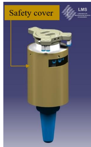
Figure 77: Safety cover for flexible gripper
