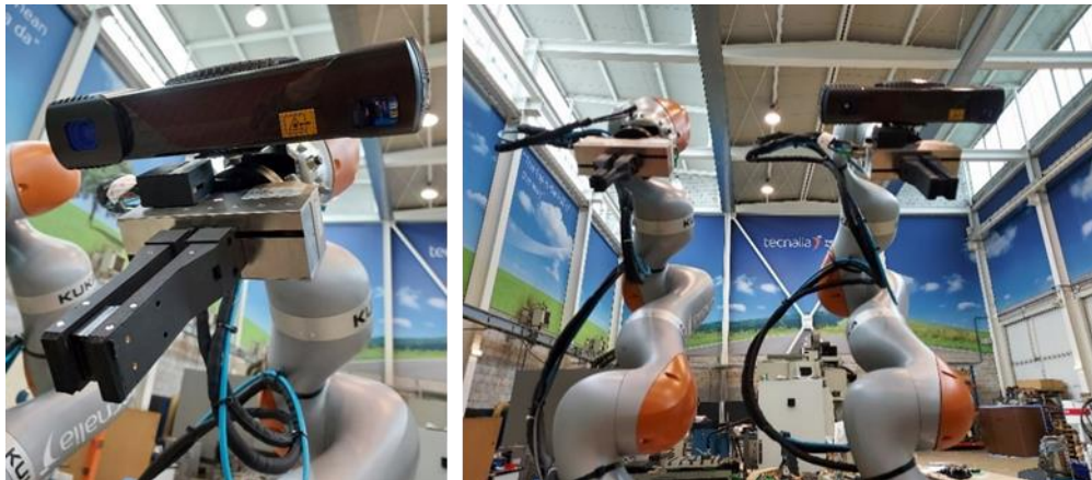
Figure 68: 3D sensor eye-in-hand configuration
